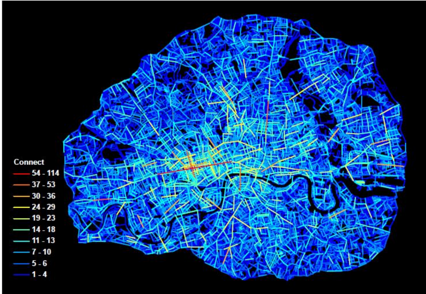
Fig. 1 – Ten hierarchical levels for the London open space represented by the axial lines; the reddish lines constitute a part of the London mental map.
