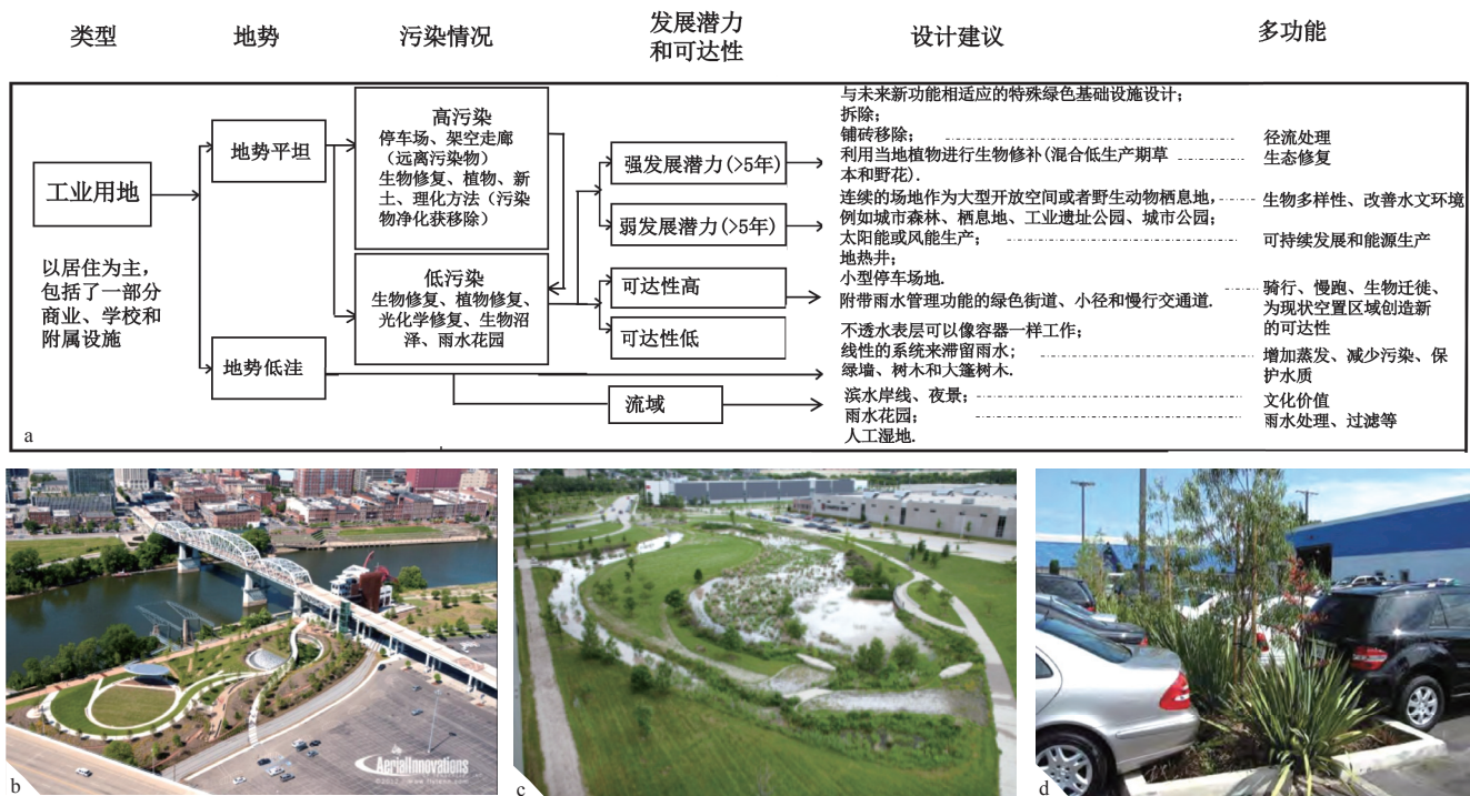
图2 工业用地绿色基础设施设计流程图 (a.流程图, b.坎伯兰公园: 水槽不允许雨水渗入地下, 而是从公园、毗邻的运动场和桥梁收集水并回收灌溉和景观 [32] , c.MVIC雨水公园, 管理雨水径流的同时提供一个新的公共空间, d.在加利福尼亚圣莫尼卡市的停车场的洼地生物渗透 [33] ) Fig.2 design flowchart for industrial areas and attached infrastructure (a.flowchart b.a view of Cumberland Park, Nashville, TN c.the MVIC Storm water Park manages storm water runoff while providing a new public space with a pedestrian and bicycle trail d.the parking lots in the city of Santa Monica, California: parking lot swales to bio-infiltrate before becoming a commercial site)
