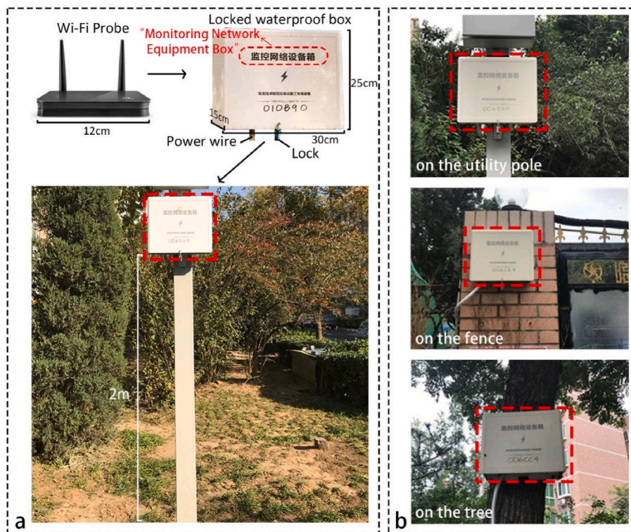
Fig. 4. The demonstration of the integrated Wi-Fi device box (a) and its installation (b).
