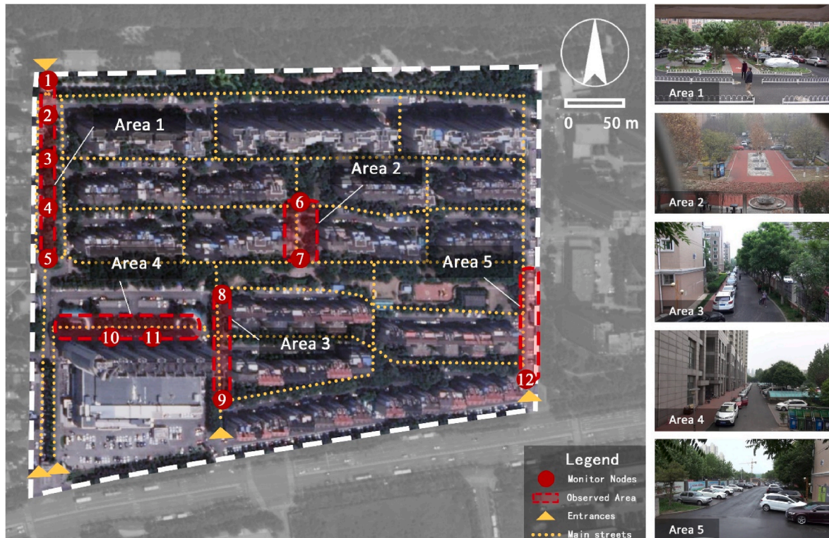
Fig. 13. The installation location of Wi-Fi probes and the observed areas in the field observation.
