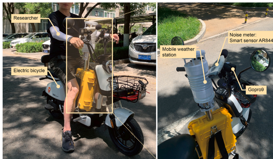
Fig. 4. Descriptions of the e-bike carrying professional monitoring devices.
