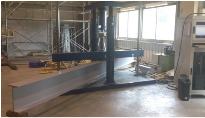
Figure 1. A 6 m span length of H410-L6
